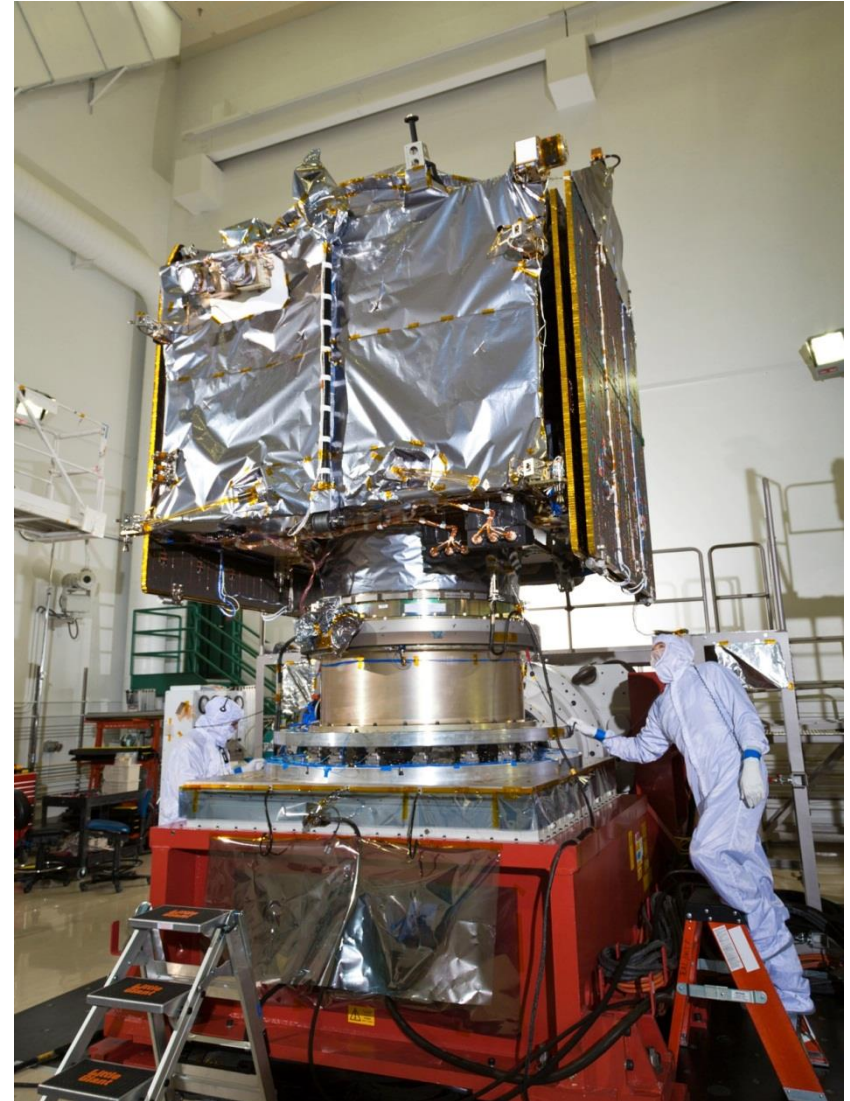
MAVEN on Shaker – Sine Vibration
