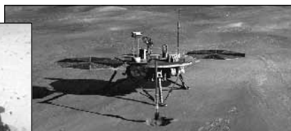
The 2007 Phoenix Mission will use a robotic arm to dig into the ice at the Martian north pole.
